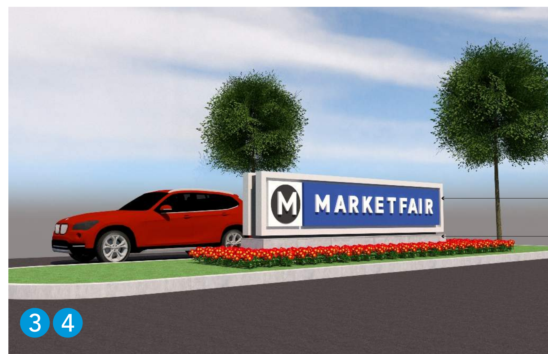
3 4 Proposed Replacement Monument Sign Elevation (Opposite Side Is Similar) (Internally Illuminated) Scale: 3/8" = 1'-0"
