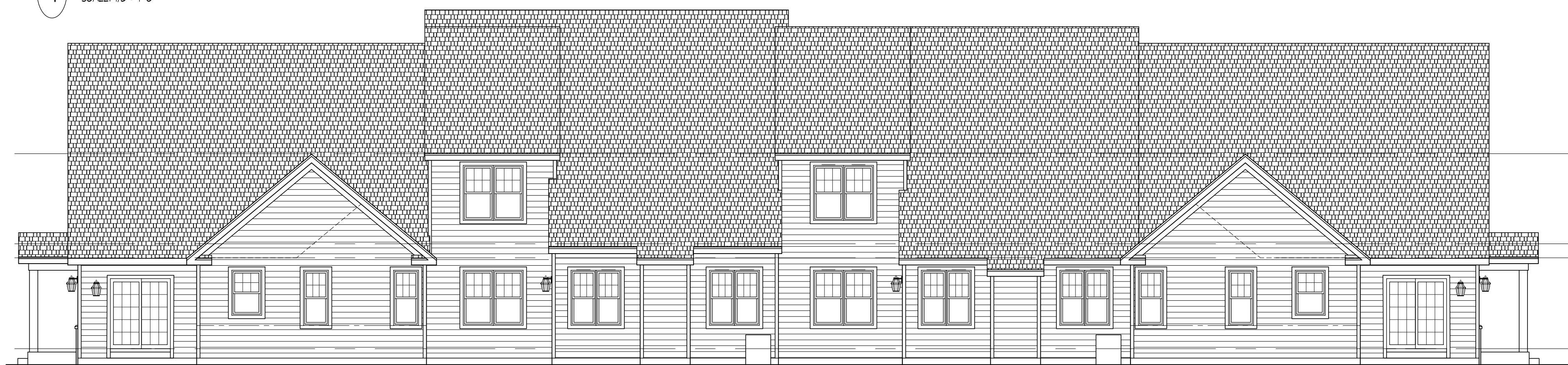
5 BUILDING TYPE D - REAR ELEVATION - STYLE 2 SCALE: 1/8" = 1'-0"
