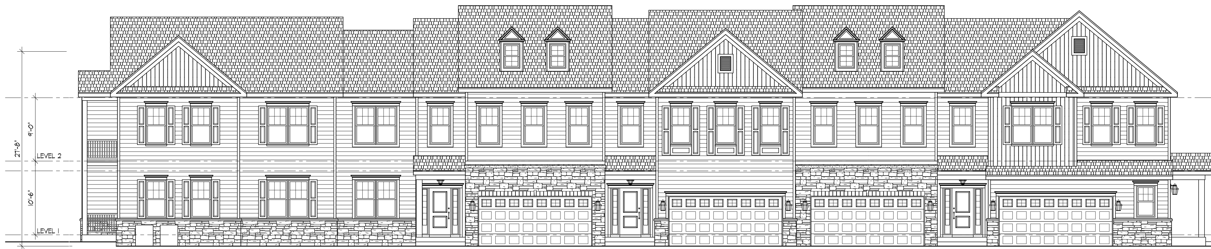
1 AFFORDABLE (FRONT AND REAR) MODEL B MODEL B MODEL B MODEL A BUILDING TYPE E - FRONT ELEVATION - STYLE 1 SCALE: 1/8" = 1'-0"
